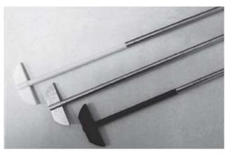
Figure. Examples of Apparatus 2 paddles.
