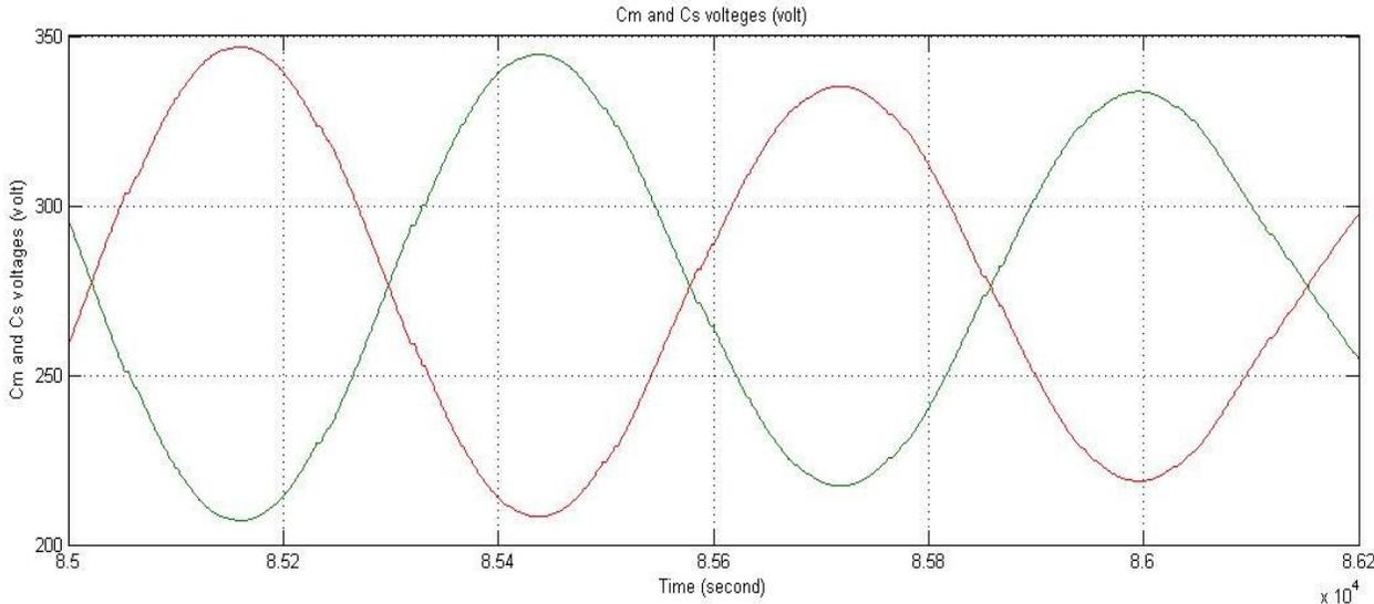
Fig3.4 Capacitor Cm and Cs Voltages Waveform
