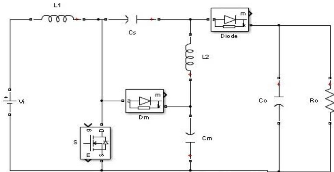
Fig 2.1 Modified SEPIC converter
