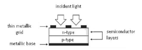
Fig-1.1 Basic PV Cell Structure
