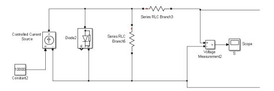
Fig-2.2 PV cell equivalent circuit
