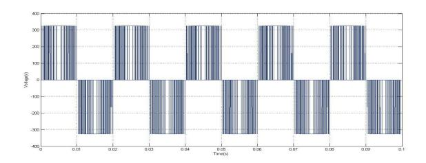
Fig-3.6 Inverter output voltage
