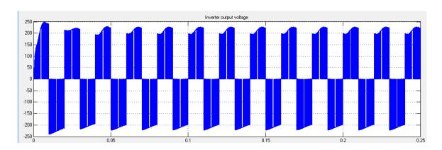
Fig-3.9 output voltage waveform (without filter)
