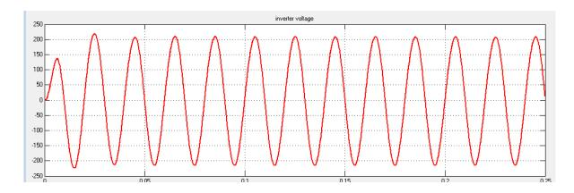
Fig-3.10 output voltage waveform (with filter)
