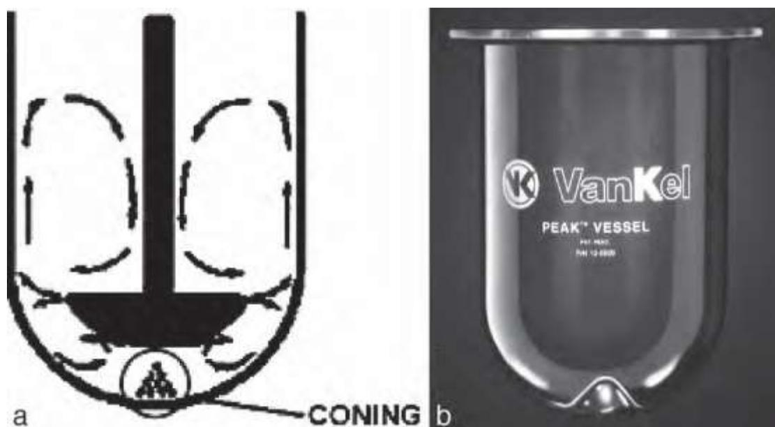
Figure. Cone formation (12a) and Peak vessel configuration (12b).
