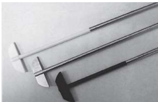
*Figure. Examples of Apparatus 2 paddles.*
