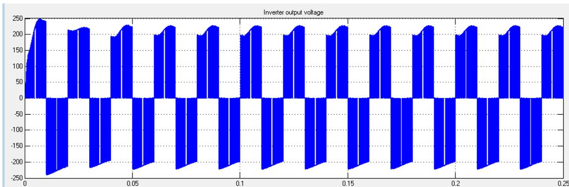
Fig-3.9 output voltage waveform (without filter)
