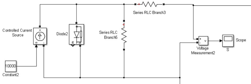
Fig-2.2 PV cell equivalent circuit
