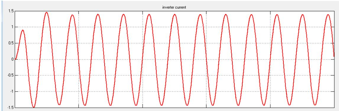
Fig-3.8 output current waveform (with filter)
