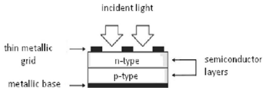
Fig-1.1 Basic PV Cell Structure
