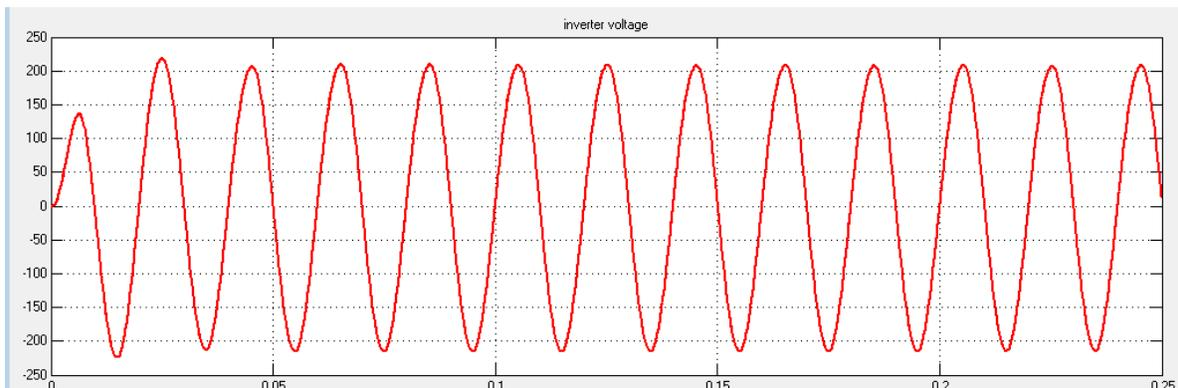
Fig-3.10 output voltage waveform (with filter)
