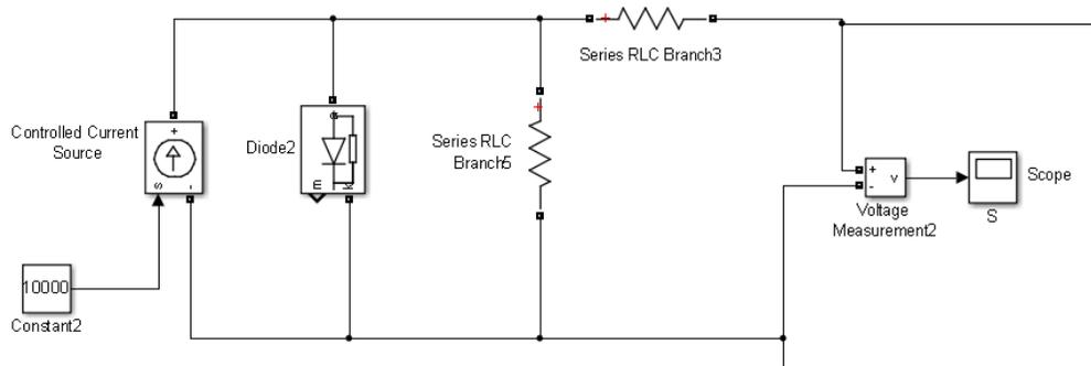
Fig-2.2 PV cell equivalent circuit
