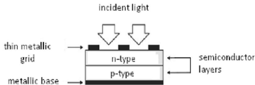
Fig-1.1 Basic PV Cell Structure
