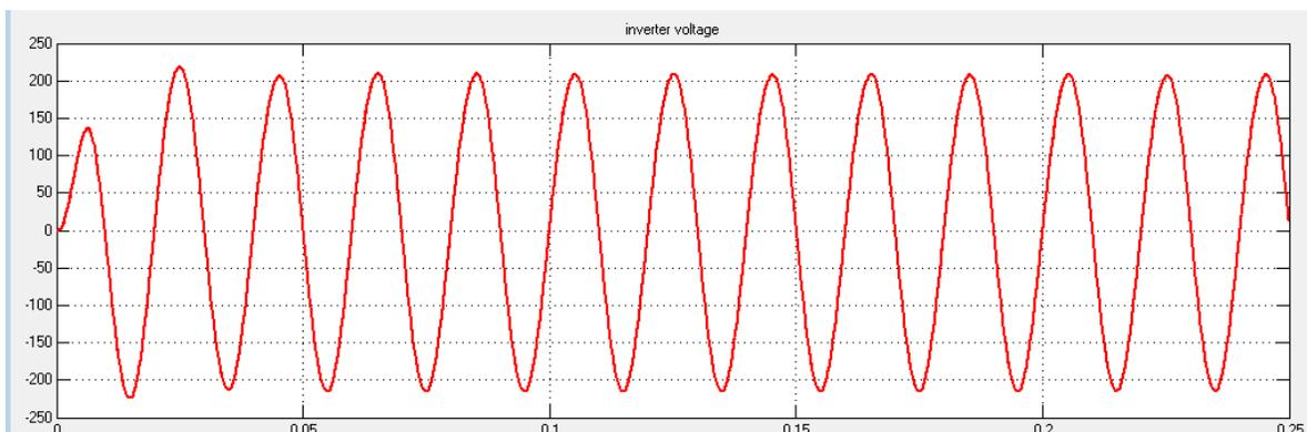
Fig-3.10 output voltage waveform (with filter)
