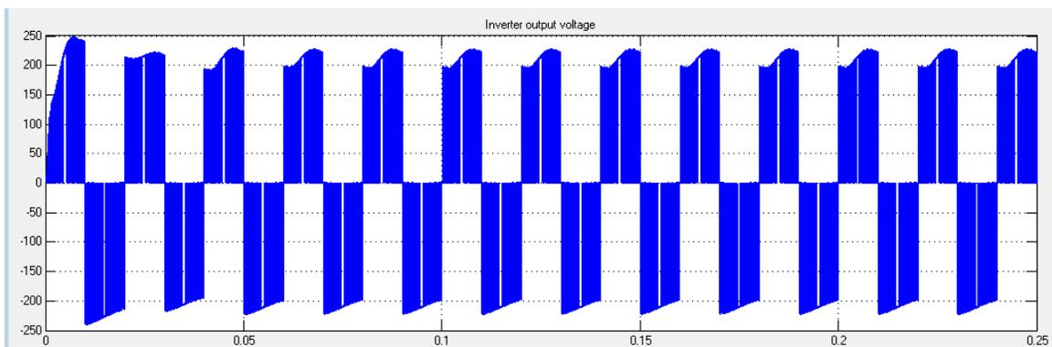
Fig-3.9 output voltage waveform (without filter)
