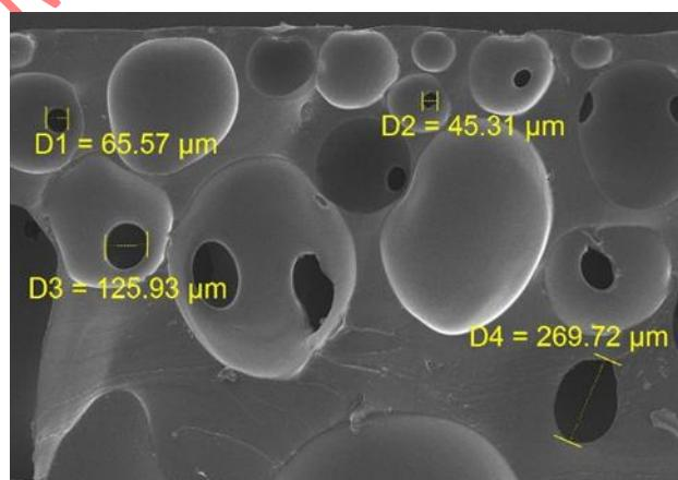
Fig. 2. SEM micrograph showing the microporous surface of the folate-polymer composite sample (500  $\mu\text{m}$  scale bar).
