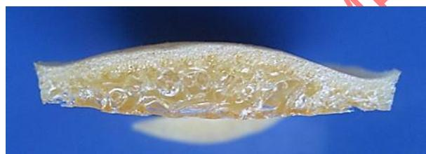
Fig. 1. Macrograph of microporous structure of the folate-polymer composite sample
